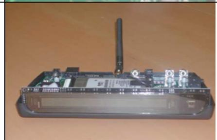
11. Carefully install the top of the case, making sure that the display module and the lens fit into the tabs in the top of the case. Hold the two halves of the case together while turning the unit over to install the screws. **Do not over tighten the screws!** They only require a small amount of torque.
