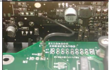
10. Reinsert the lens in the front of the case. Make sure it is centered, and resting between the two small plastic stops on either side of the window. Before installing the top of the case, **make sure that the cables are clear** from the two holes in the front of the circuit board. These holes line up with the mounting posts in the top of the case. Push the cables a little to the side if they are in the way.
