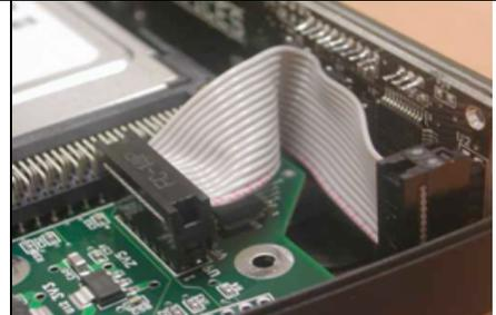
9. Attach the jumper lead by sliding the connector down onto the pin.
